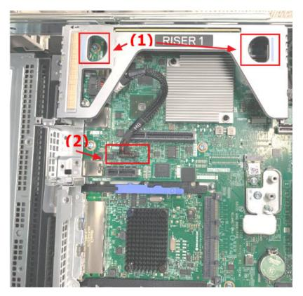
**c.** Open the card retention latch and remove the slot cover of an empty PCIe slot
