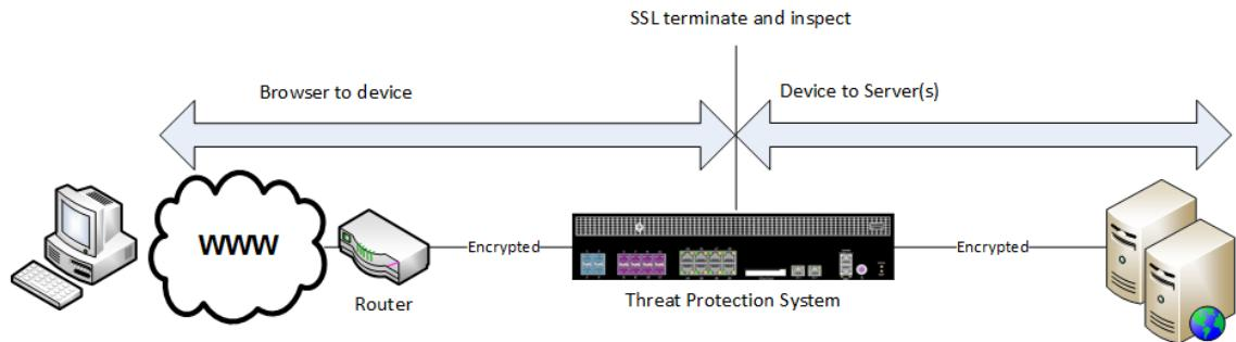
With access to the server certificate and private key, the TPS is a transparent proxy that receives and decrypts SSL data, inspects it using the Threat Suppression Engine, and then encrypts it before sending it to the actual destination.
