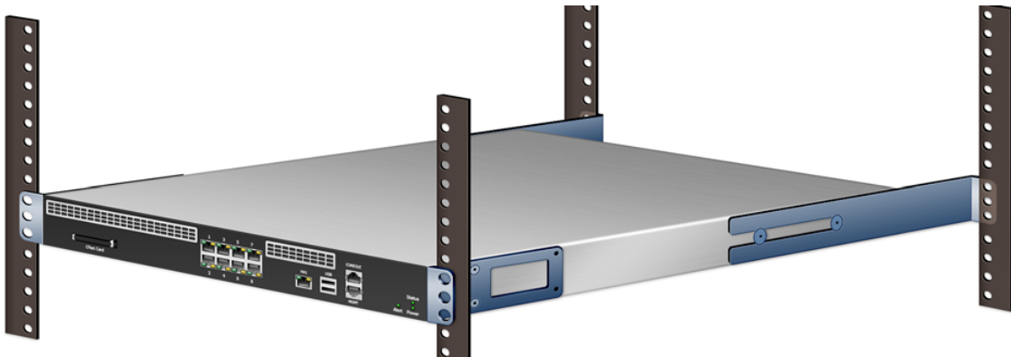
Figure 1-4 1U chassis in a four-post rack
