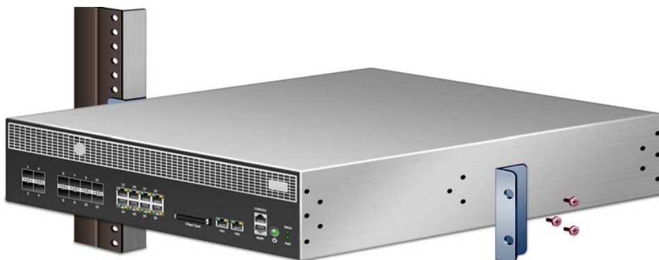
Figure 1-7 2U chassis with mid-mounting in a two-post rack
