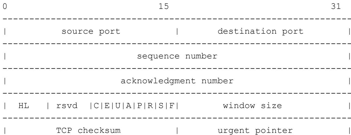
A TCP header usually holds 20 octets of data, unless options are present. The first line of the graph contains octets 0 - 3, the second line shows octets 4 - 7 etc.
