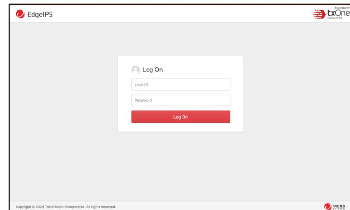
Before connecting the PC/Laptop to EdgeIPS, the PC's IP address should be set to 192.168.127.100. After that, connect the PC and EdgeIPS using an Ethernet cable. Open a web browser on your PC and type “https://192.168.127.254” into the address bar. A pop-up window will open to ask for user name and password. Please type the default username, “admin”, and password, “txone”.
