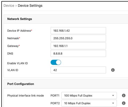
The screenshot shows the 'Device > Device Settings' interface. Under 'Network Settings', the 'Device IP Address' is set to 192.168.1.42, 'Netmask' to 255.255.255.0, 'Gateway' to 192.168.1.1, 'DNS' to 8.8.8.8, and 'Enable VLAN ID' is turned on with 'VLAN ID' set to 42. Under 'Port Configuration', 'Physical interface link mode' for 'PORT1' is set to '100 Mbps Full Duplex' and for 'PORT2' to '10 Mbps Full Duplex'.
