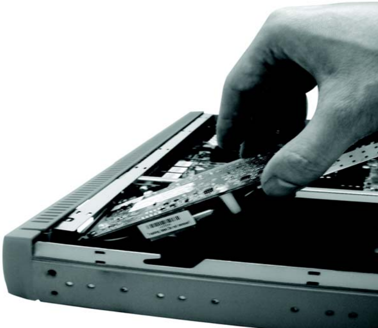
FIGURE 1-35. Slide the card to the front of the device
