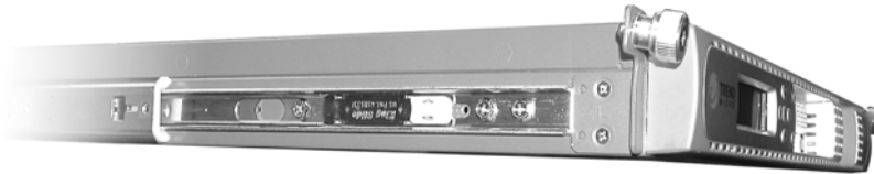
FIGURE 1-13. Completed rack ear and rail preparation
