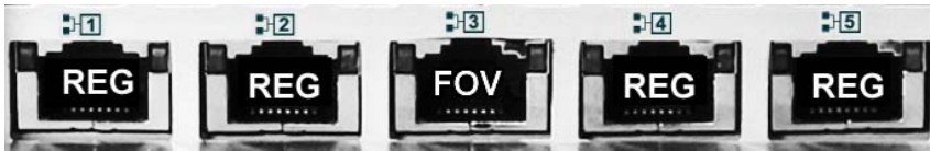
FIGURE 3-11. Interface allocation for a port grouping with failover deployment
