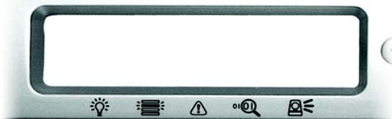
FIGURE 1-3. POWER, UID, SYSTEM, POLICY, and OUTBREAK LED indicators
