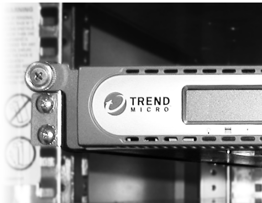
FIGURE 1-26. Mounted Network VirusWall Enforcer 2500 device (fixed mount)
