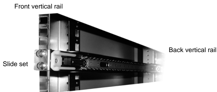
FIGURE 1-15. A slide set installed in a four-post rack
