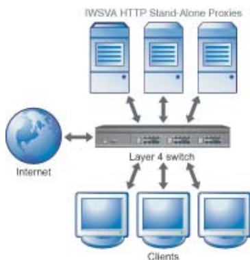
FIGURE 7-4. Forward proxy with transparency
