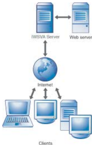
FIGURE 7-5. Reverse proxy protects Web server from clients
