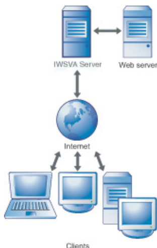
FIGURE 5-5. Reverse proxy protects Web server from clients
