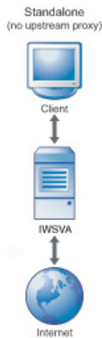
FIGURE 5-2. Forward, no upstream proxy
