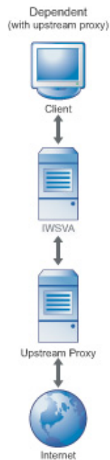
FIGURE 5-3. Forward, upstream proxy
