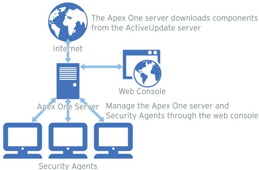
**FIGURE 1-1. How the Apex One server works**
