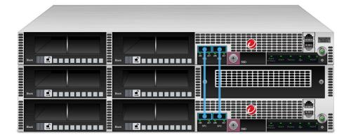
The next example shows the network I/O modules are properly installed in slots 1 and 2 of the network segment device (bottom).
