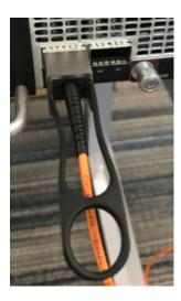
The next example shows a special purpose port with the AOC cable partially inserted upside down.
