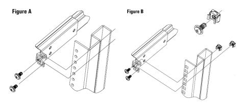
5. Attach the inner section of the slide rail to the device chassis.
