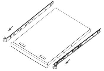
6. Slide the chassis into the rails.
