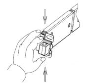
2. Press the white latch on the inner section of the slide and pull to remove that section.
