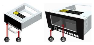
To remove the blank module, slide the slide latch (1) to the right and pull on the handle (2 on left module) or grab point (2 on right module).
