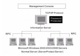
FIGURE 1-1. ServerProtect Three-tier Architecture
