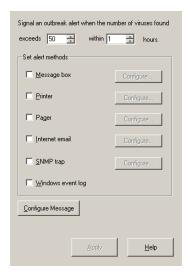
FIGURE 3-58. ServerProtect Outbreak Alert Events Configuration Window
