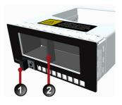
To remove the blank module, slide the slide latch (1) to the right and pull on the handle (2 on left module) or grab point (2 on right module).
