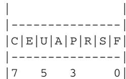
These are the TCP control bits we are interested in. We have numbered the bits in this octet from 0 to 7, right to left, so the PSH bit is bit number 3, while the URG bit is number 5.
