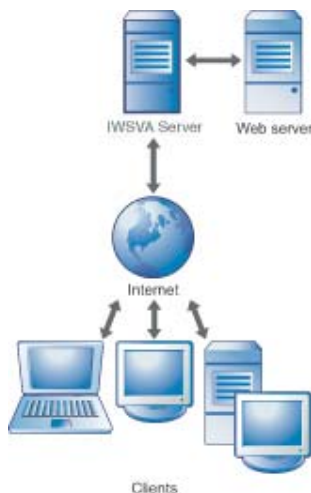
FIGURE 3-5 Reverse proxy protects Web server from clients
