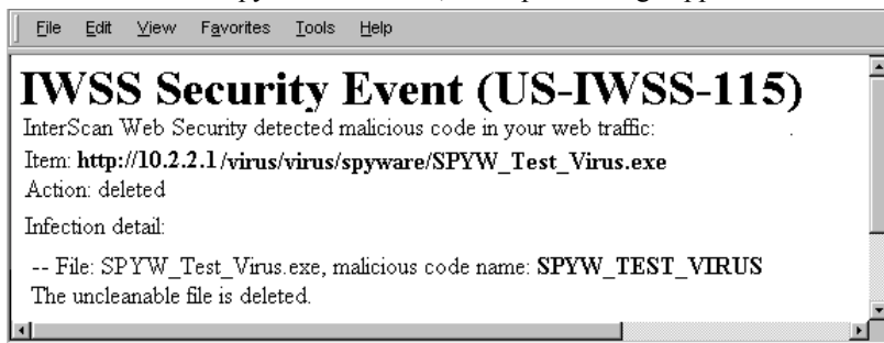
FIGURE D-6 A sample message after detecting a spyware with action “Delete” setting.
