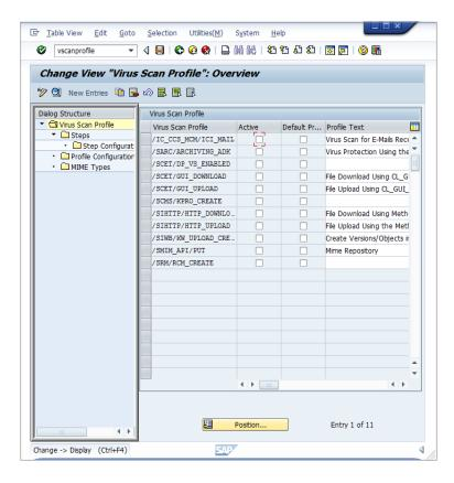
2. In Edit mode, click **New Entries**. The virus scan profiles will define how specific transactions (file uploads, file downloads, etc.) are handled corresponding to the virus scan interface. To have the previously configured virus scan adapter used in the application server, a new virus scan profile needs to be created:
