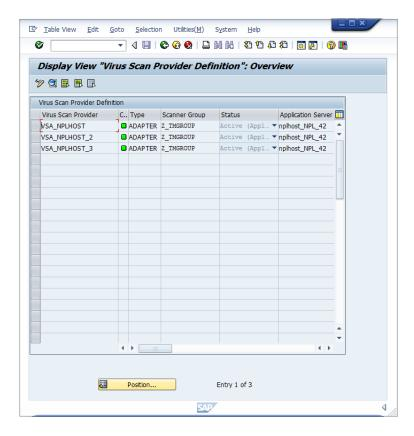
At this point, the VSI configuration is nearly finished. The application server is now ready to process file transactions using a virus scan provided by Trend Micro Deep Security.
