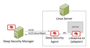
Deep Security Manager connects with the Deep Security Agent located on the SAP NetWeaver Linux server. The Agent connects with libsapvsa.so, which is the virus adapter provided by Trend Micro for scanning purposes.
